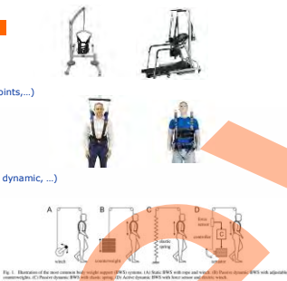
Fig. 1. Representation of the four main types of BWS systems: (A) Static BWS with one pole and one (B) Static BWS with two poles and one (C) Dynamic BWS with one pole and one (D) Dynamic BWS with two poles and one
