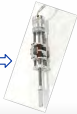
Series Elastic Actuator
