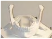
3D printed mandible based on segmented CT image
